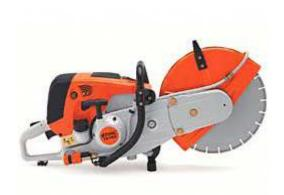
Very powerful 5.0 kW engine with 350 mm cutting wheel. Includes a long life air filter system with cyclone air routing. Ergonomic design with optimised handling positions. ElastoStart plus, compensator and decompression valve. Water attachment and composite cutting wheel come as standard. Can be operated by hand or mounted on a FW 20 cart.
