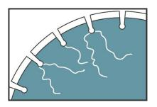
Excessive cutting pressure or the metal bond is too hard for the material being cut causing the blade to pound in the cut. Metal fatigue will eventually cause the core to crack. Use a blade with a softer bond
