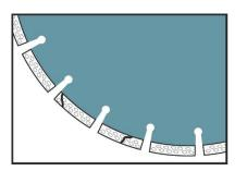
Excessive cutting pressure or the metal bond is too hard for the material being cut causing the blade to pound in the cut. Use a blade with a softer bond
